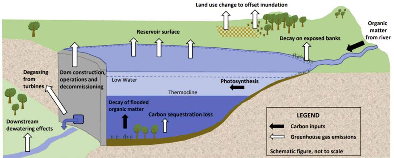
Figure 1: Emissions pathways in a hydropower facility included in All-Res.
